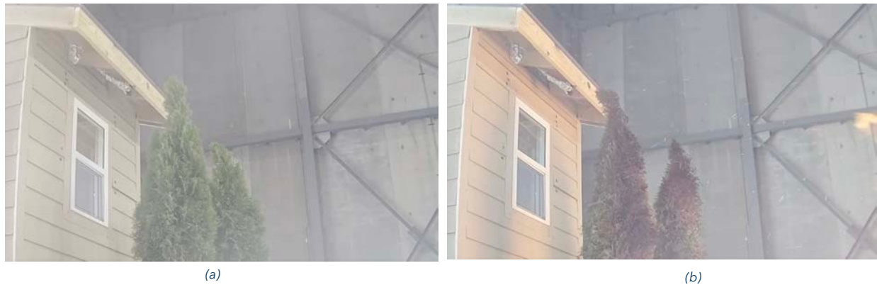
Figure 7. Effect of the heat exposure on drying well-hydrated vegetation. (a) Close-up of the shrubs at the beginning of the experiment, showing them fully hydrated. (b) Close-up 13 minutes after ignition of the cribs, showing the shrubs have dried out just before ignition.
