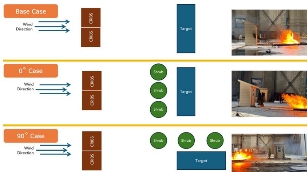
Figure 3. Experimental setup for each of the 3 scenarios including a photo of the configuration.
