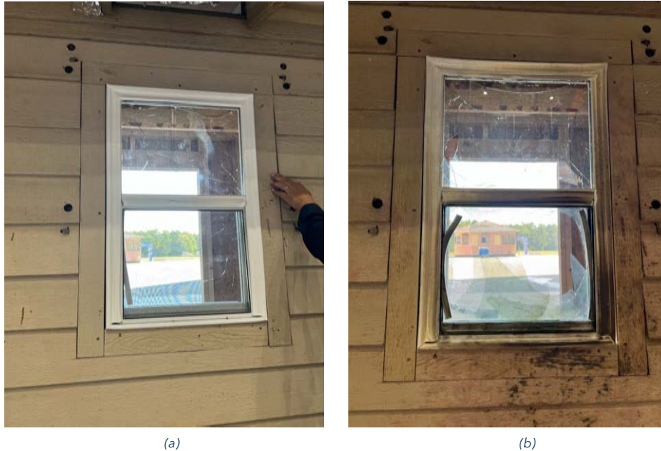
Figure 4. Example of the increased damage when shrubs are present. (a) shows the cracked windowpane damage from the base case without shrubs. (b) shows the damage amplification when shrubs were present including discoloration to the siding and the broken windowpane. In (b), the missing pieces of glass in the broken window create an opening in the building envelope for flames and embers to enter the structure.
