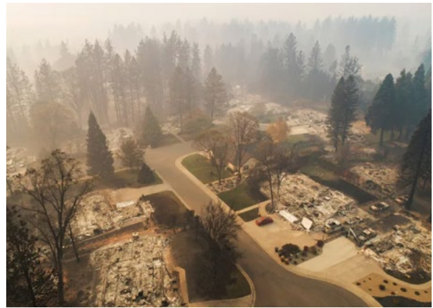
Home destruction with adjacent unconsumed shrub and tree vegetation, Paradise (Image: LiPo Ching/Bay Area News Group)
